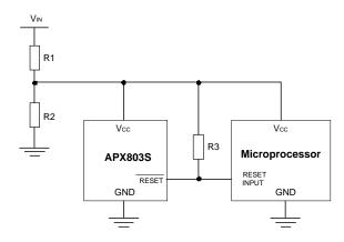
When  $V_{CC}$  just rises up to the  $V_{TH}$  value (2.93V in this case), the internal oscillator will start working, which may pull some considerable current from the source voltage, such as  $60\mu$ A or so. Take above topology as real application example, below equation required to meet to make sure the IC boot up smoothly. Given  $V_{CC} = 13.2$ V and R3 =  $100k\Omega$ , an appropriate R1/R2 value combination would be R1 =  $15.6k\Omega$  and R2 =  $7.3k\Omega$ .
