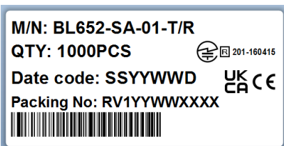
Figure 17: BL652 Product Identifier Labels for Reel, Bag, and Box (BL652-SA-01-T/R in the exemplary photo)
