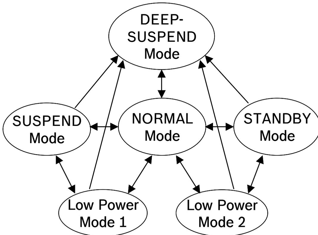
Figure 2: Power mode transition diagram
