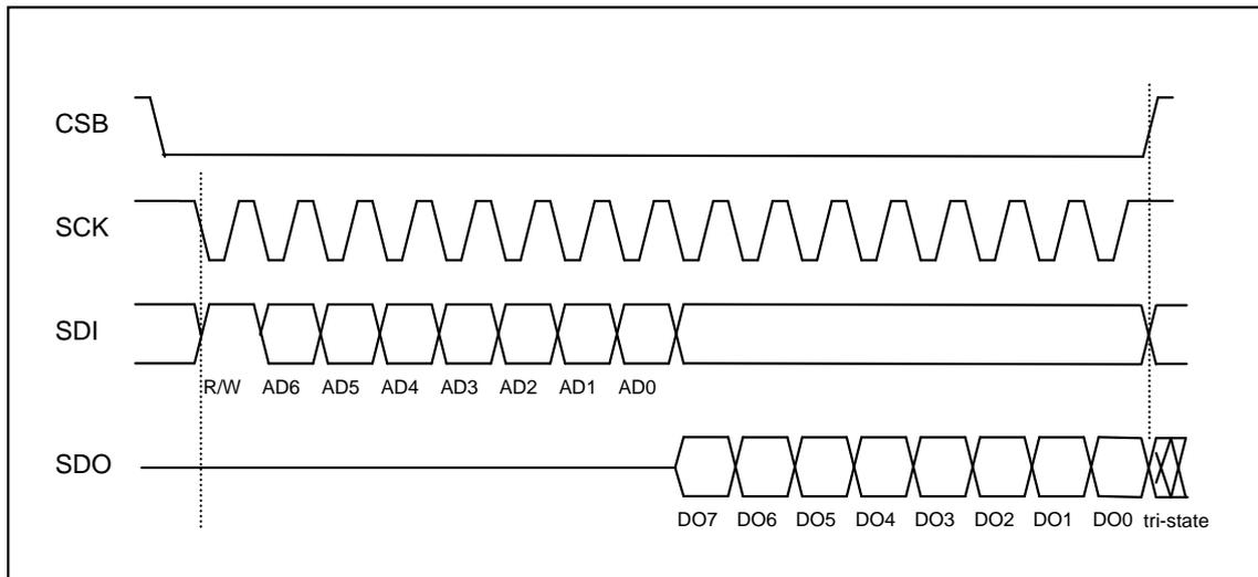
Figure 28: 4-wire basic SPI read sequence (mode '11')
