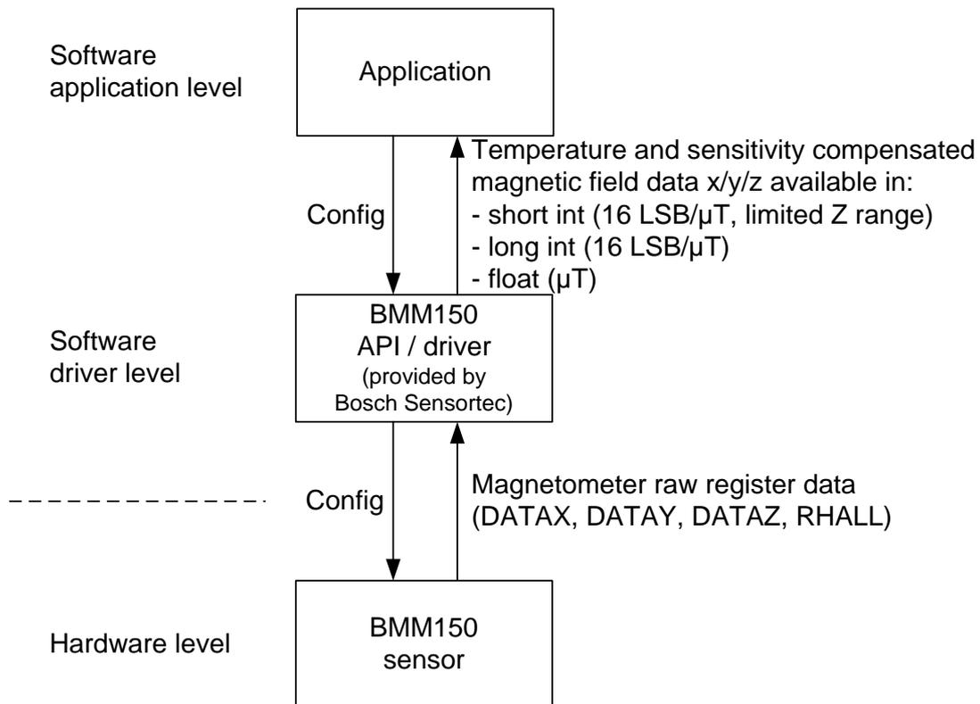
Figure 21: Calculation flow of magnetic field data from raw magnetometer register data
