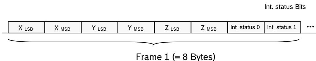
If only one axis is enabled (and tag is disabled), the format of the data read-out from register fifo\_data<7:0> is as follows (example shown: Y-axis only, other axis are equivalent). The buffer depth of the FIFO is independent of the fact whether all or a single axis have been selected.
