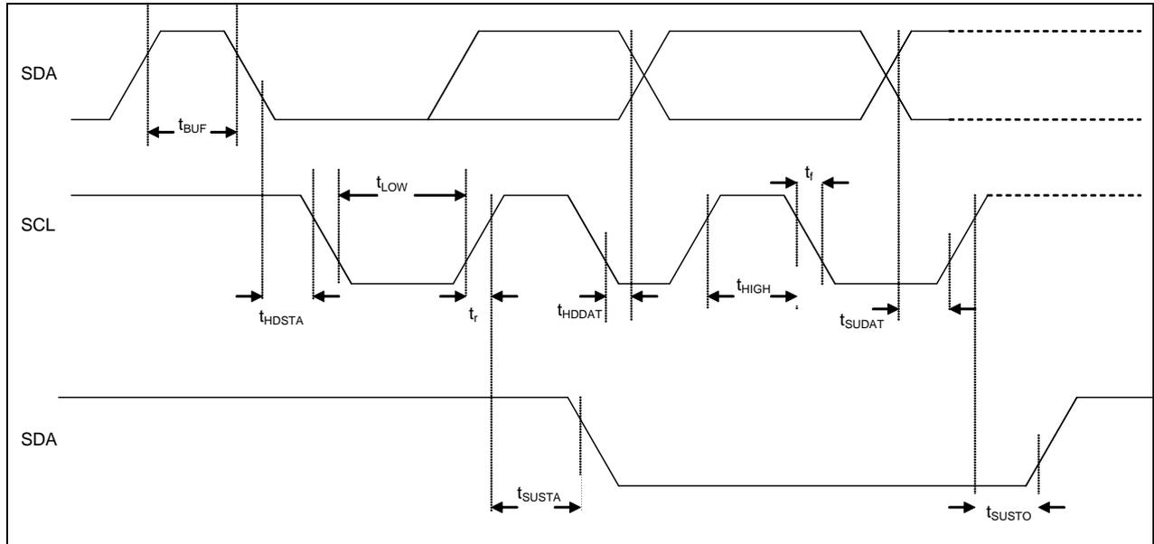
Figure 31: I<sup>2</sup>C timing diagram
