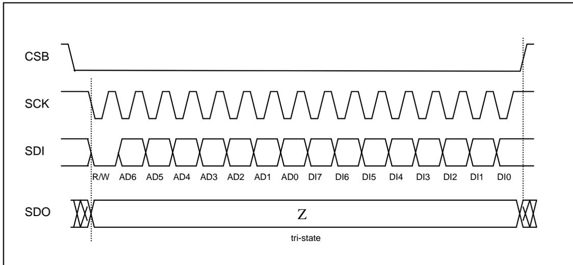
Figure 27: 4-wire basic SPI write sequence (mode '11')
