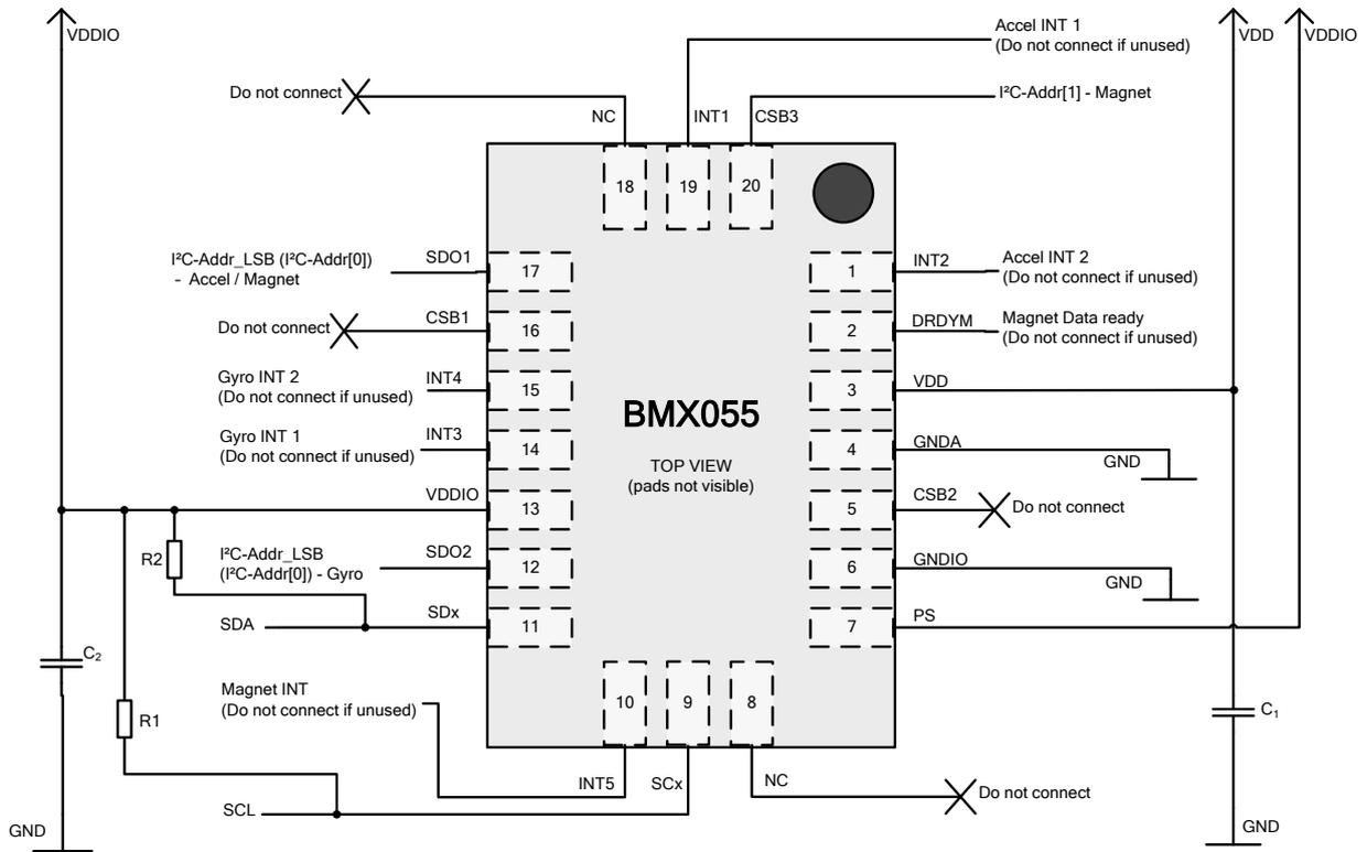
Figure 39: I<sup>2</sup>C connection
