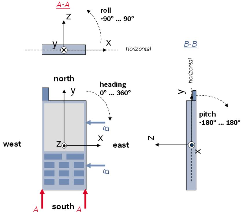
Figure 43: Heading, pitch and roll in Android coordinate frame
