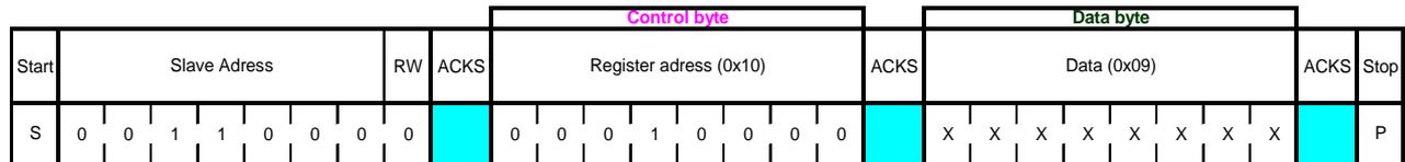
Figure 32: I<sup>2</sup>C write
