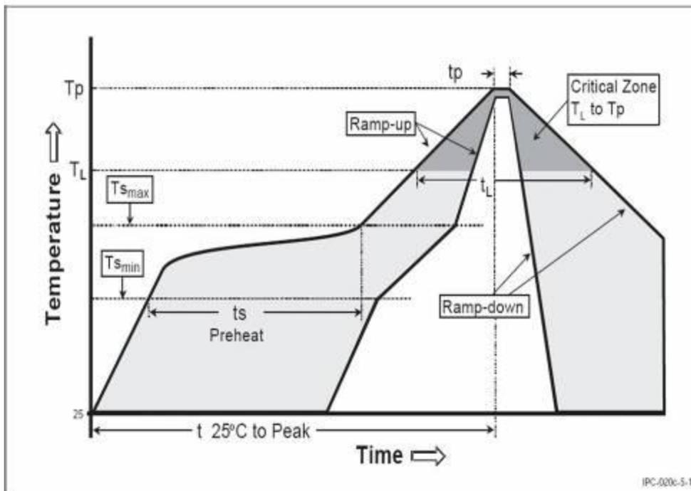
Figure 45: Soldering profile recommendation
