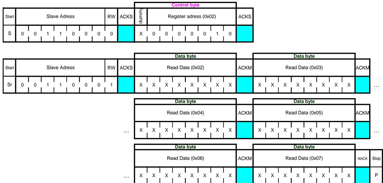
Figure 33: I<sup>2</sup>C multiple read
