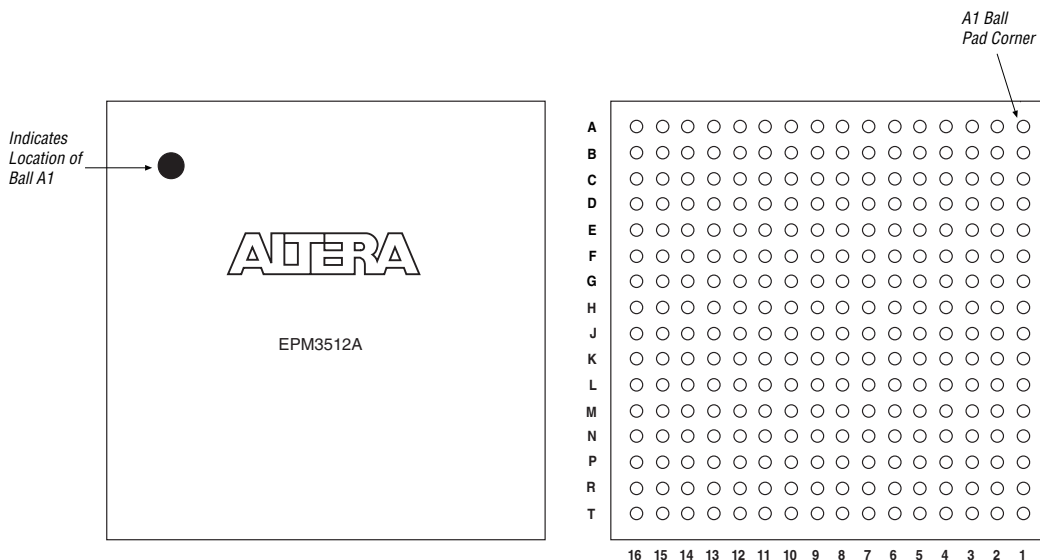
Figure 18. 256-Pin FineLine BGA Package Pin-Out Diagram
