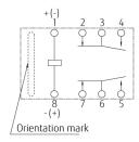
PC board mounting hole layout (BOTTOM VIEW)
