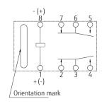
PC board mounting pad layout (TOP VIEW)
