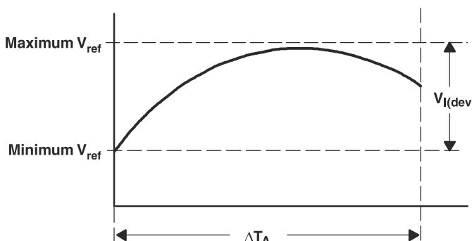
$\alpha_{V_{ref}}$  is positive or negative, depending on whether minimum  $V_{ref}$  or maximum  $V_{ref}$ , respectively, occurs at the lower temperature. The full-range temperature coefficient is an average and therefore any subsection of the rated operating temperature range can yield a value that is greater or less than the average. For more details on temperature coefficient, refer to the [Voltage Reference Selection Basics White Paper](#).
