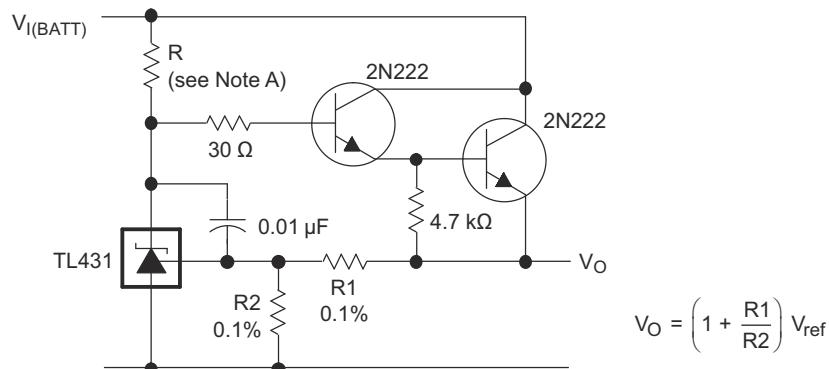
A. R should provide cathode current  $\geq 1\text{mA}$  to the TL431 at minimum  $V_{(BATT)}$ .
