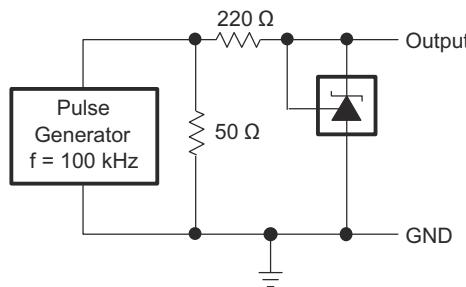
Figure 6-15. Test Circuit for Pulse Response
