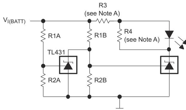
$$\text{Low Limit} = \left(1 + \frac{R1B}{R2B}\right)V_{\text{ref}}$$
