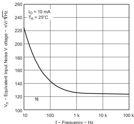
**Figure 6-7. Equivalent Input Noise Voltage vs Frequency**
