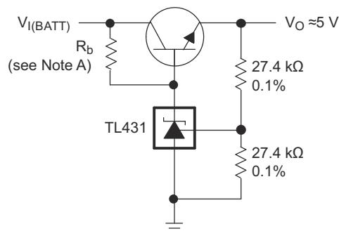
A.  $R_b$  should provide cathode current  $\geq 1\text{mA}$  to the TL431.
