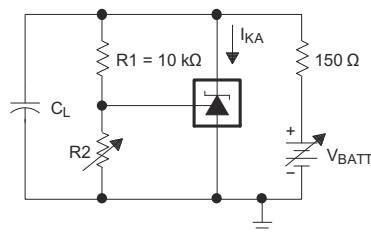
Figure 6-17. Test Circuits for Stability Boundary Conditions
