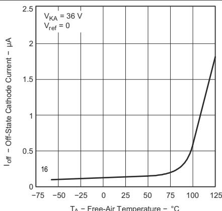
**Figure 6-5. Off-State Cathode Current vs Free-Air Temperature**
