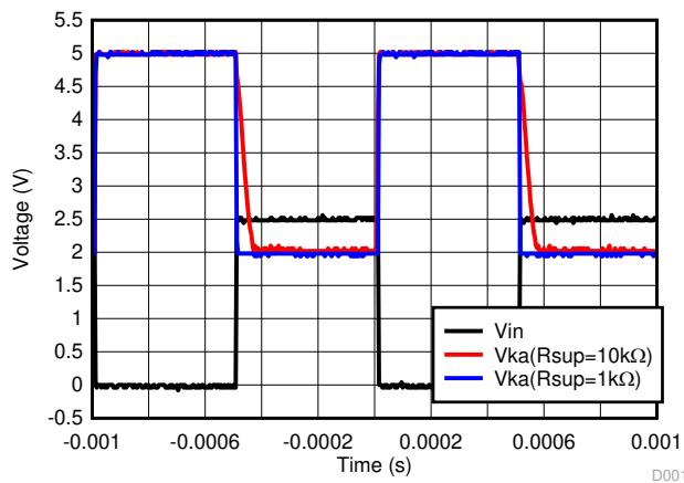
**Figure 9-2. Output Response With Various Cathode Currents**
