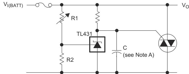
A. Refer to the stability boundary conditions in [Figure 6-16](#) and [Figure 6-18](#) to determine allowable values for C.
