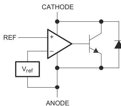
**Figure 8-1. Equivalent Schematic**
