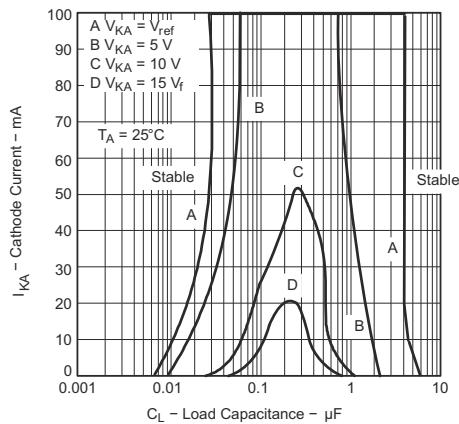
The areas under the curves represent conditions that can cause the device to oscillate. For curves B, C, and D,  $R_2$  and  $V^+$  are adjusted to establish the initial  $V_{KA}$  and  $I_{KA}$  conditions, with  $C_L = 0$ .  $V_BATT$  and  $C_L$  then are adjusted to determine the ranges of stability.
