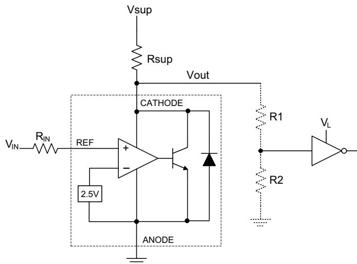
Figure 9-1. Comparator Application Schematic
