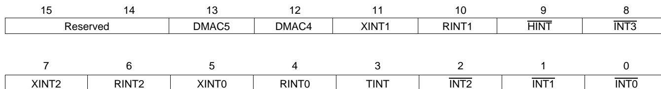
Figure 3-23. IFR and IMR Registers
