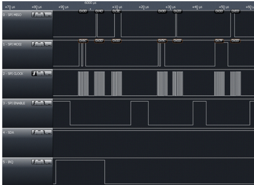
Figure 6-24. IRQ With One Byte in FIFO
