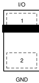
Figure 5-1. DPY Package 2-Pin X1SON Top View
