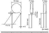
Lead Code Coating Extension e A2. A3 Up to the end of crimp 0.6±0.05 Fia. 1 [Bulk] 3.0 max 0.5±0.05 Fig. 2 Vertical Crimp Long (Fig. 1) C1, CD Straight Long (Fig. 2) 3.0 max 0.6±0.05 Fig. 2 C3
