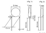
Lead Code | Coating Extension e Style ø d A2, A3, A4 Up to the end of crimp 3.0 max 0.6±0.05 Fig. 2
