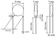
[Bulk] Vertical Crimp Long (Fig. 1) Straight Long (Fig. 2)
