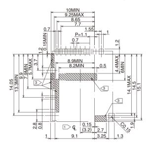
Note  $1 > \mathbf{Q}$  indicates the center line of the microSD card slot.
