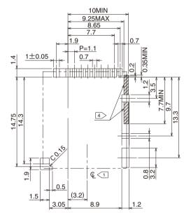
Note 1 > Q indicates the center line of the microSD card slot.
