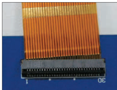
✗ Skewed FPC Insertion
