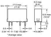
**PCB Mounting Holes** (Bottom View)
