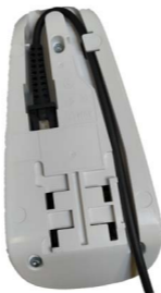
Figure 5 - Options for routing the DC cord
