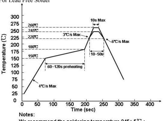
We recommend the soldering temperature 245 $\pm$ 5 $^{\circ}$ C; The maximum temperature should be limited to 260 $^{\circ}$ C.
