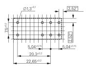
\*) With the recommended PCB hole sizes a grid pattern from 2.5mm to 2.54mm can be used.
