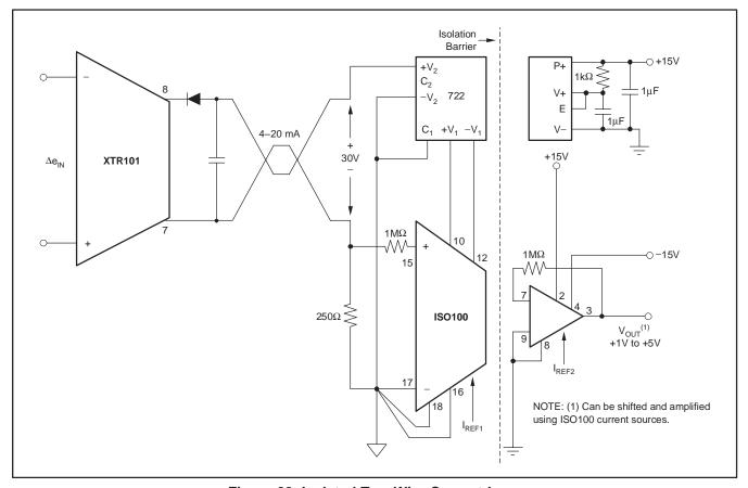
Figure 20. Isolated Two-Wire Current Loop
