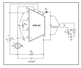
Figure 9. Circuit for Example 1
