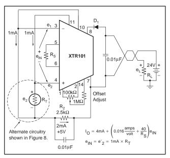
Figure 6. Basic Connection for Resistive Source
