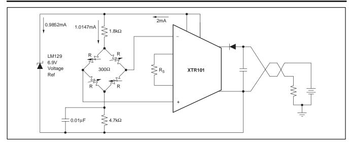
Figure 14. Bridge Input, Voltage Excitation
