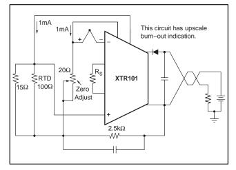
Figure 18. Thermocouple Input with RTD Cold Junction Compensation
