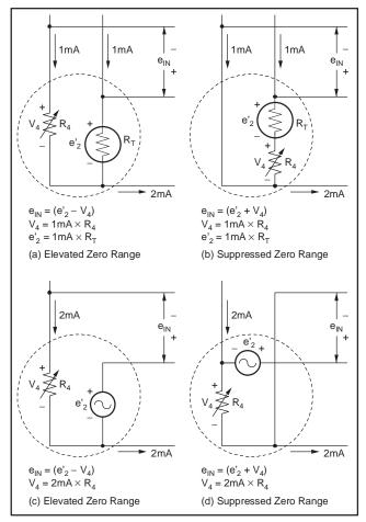
Figure 8. Elevation and Suppression Circuits
