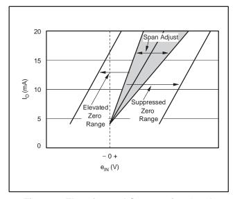
Figure 7. Elevation and Suppression Graph
