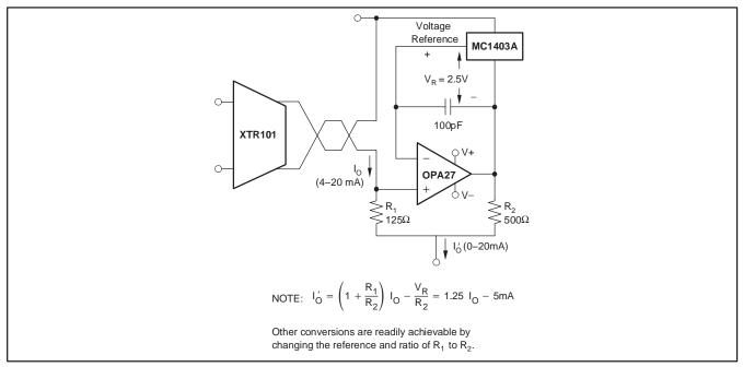
Figure 13. 0-20mA Output Converter
