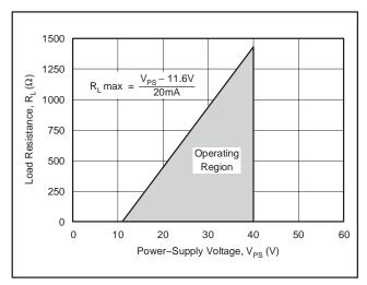
Figure 4. Power-Supply Operating Range
