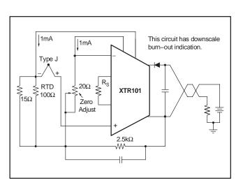
Figure 16. Thermocouple Input with RTD Cold Junction Compensation
