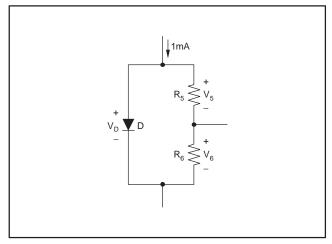
Figure 11. Cold Junction Compensation Circuit
