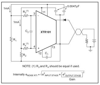
Figure 12. Optional Filtering
