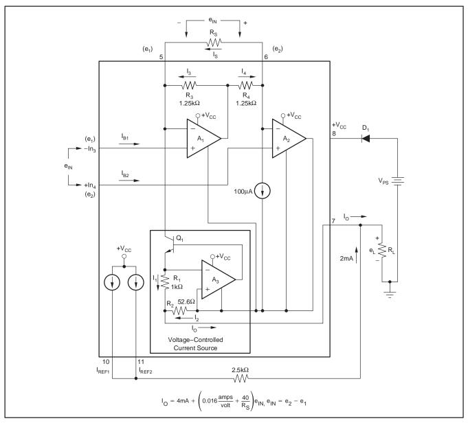
Figure 1. Simplified Schematic of the XTR101
